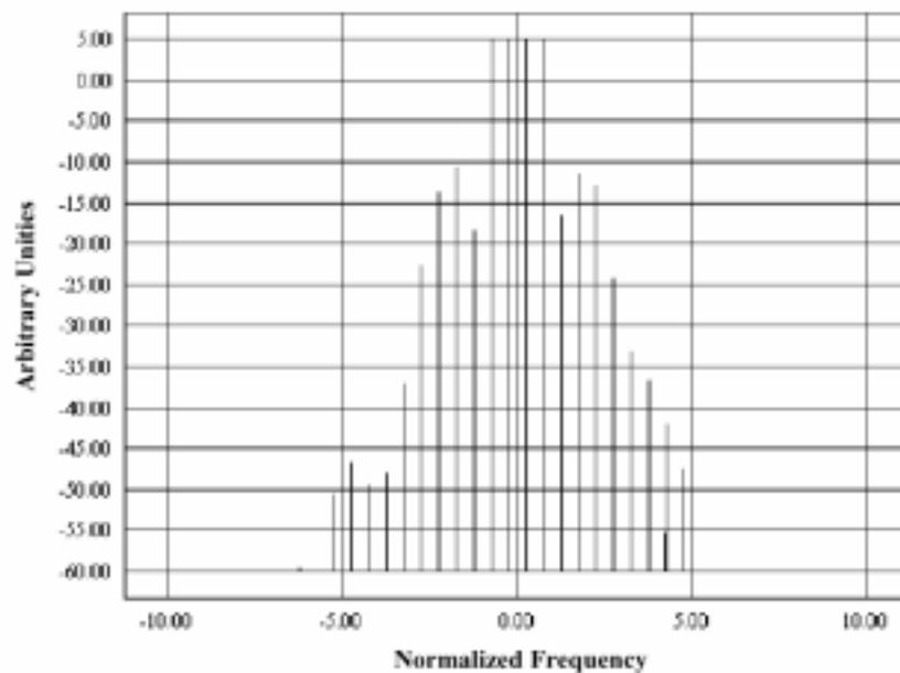
Figure 4: Frequency spectrum of the four-channel signal as calculated with the fourth-order exponential operator, using a nonlinear phaseshift  $\Delta\phi=0.05$ .
