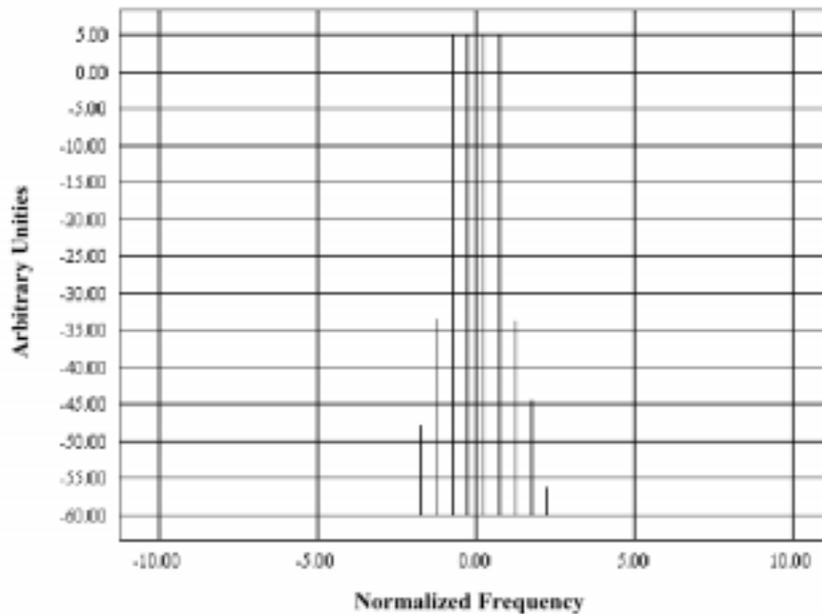
Figure 5: Frequency spectrum of the four-channel signal as calculated with the first-order exponential operator, using a nonlinear phaseshift  $\Delta\phi=0.005$ .
