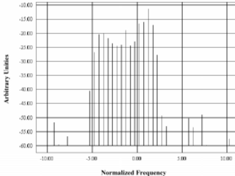
Figure 8: Frequency spectrum of the four-channel signal as calculated with the fourth-order exponential operator, using a nonlinear phaseshift  $\Delta\phi=0.01$  (after 10 km of dispersion-shifted fiber).
