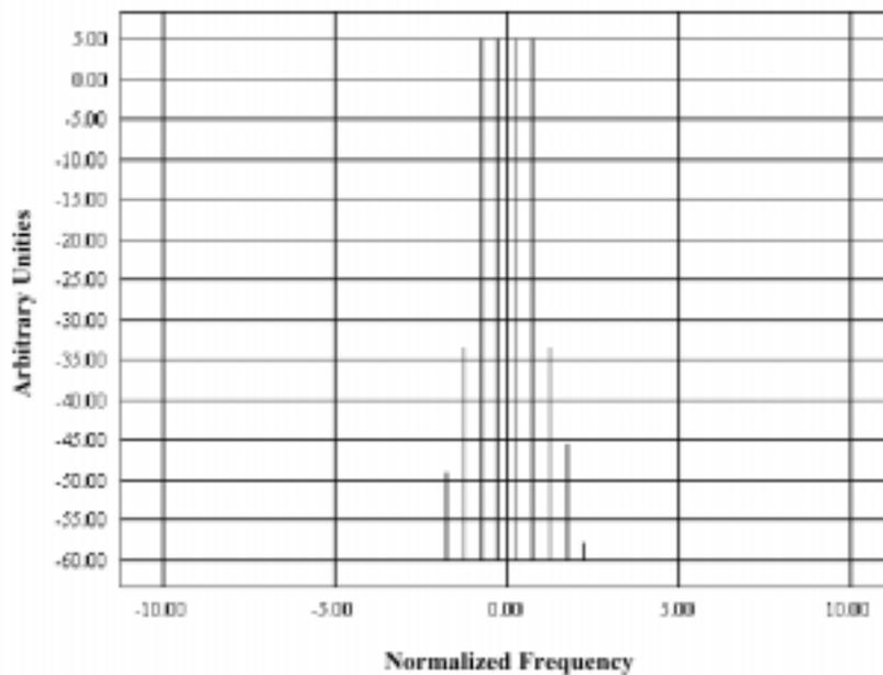
Figure 2: Frequency spectrum of the four-channel signal as calculated with the second-order exponential operator, using a nonlinear phaseshift  $\Delta\phi=0.005$ .
