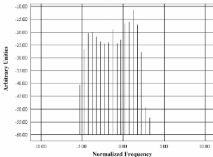
Figure 7: Frequency spectrum of the four-channel signal as calculated with the second-order exponential operator, using a nonlinear phaseshift  $\Delta\phi=0.005$  (after 10 km of dispersion-shifted fiber).
