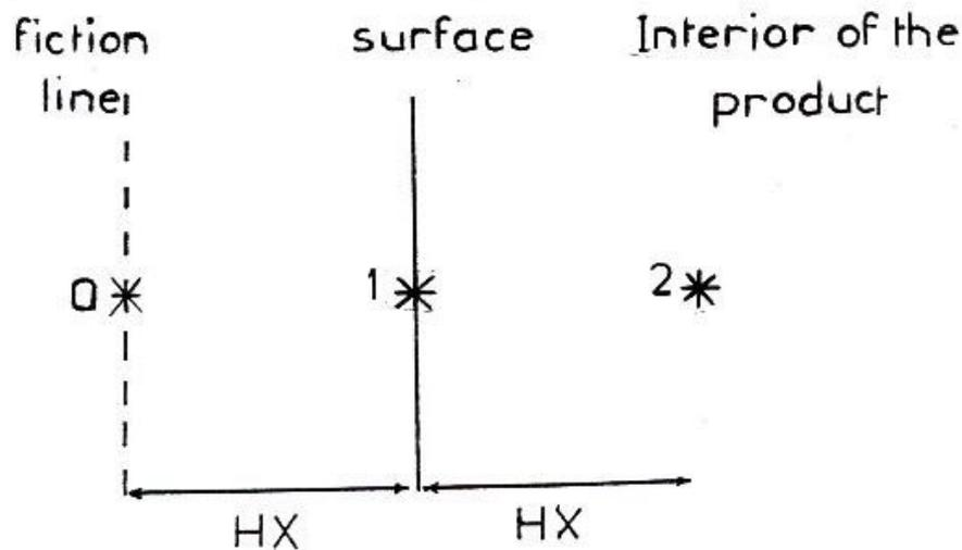
Fig.3 An example of one dimensional (x-direction) central differences between Fictitious line (point O), surface (point 1), and internal (point 2) of the processed material.
