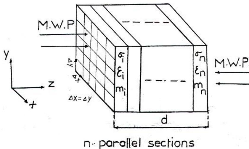
Fig.2 Processed material (cub of sand) divided into n parallel two-dimensional sections, each has specific values of ε , σ , m.
