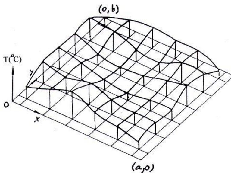
Fig. 6 Evolution of temperature  $T$  ( $^{\circ}\text{C}$ ) as a function of the system coordinates  $x$  and  $y$  for the case of conventional drying.
