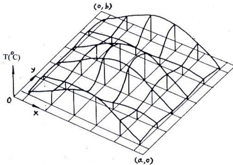
Fig. 7 Evolution of temperature T (°C) as a function of the system coordinates X and Y for the case of hybrid drying.
