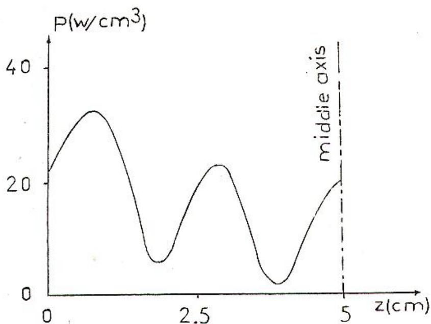
Fig. 5 Microwave drying power profile as a function of the thickness of the processed material for  $m = 15\%$ .
