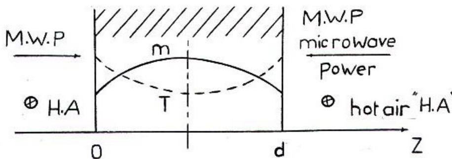
Fig. 1 General profiles for the change of humidity  $m$  and temperature  $T$  as a function of the material thickness  $d$ , for hybrid drying.
