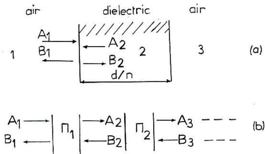
Fig. 4 Incident and reflected wave (a) for section number 1 and the chain (b) of the cub of the treated material.
