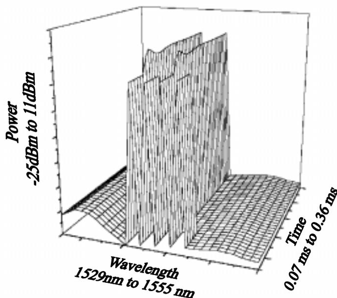
Figure 3: Temporal evolution of the signals at the output of the 12<sup>th</sup> EDFA, after dropping channels no. 2 and 4.
