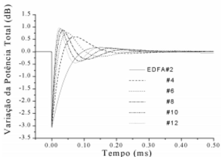
Figure 4: Variation of the total power at the output of the even-order amplifiers, when channels no. 2, 4, 6, and 8 are dropped at t=0.
