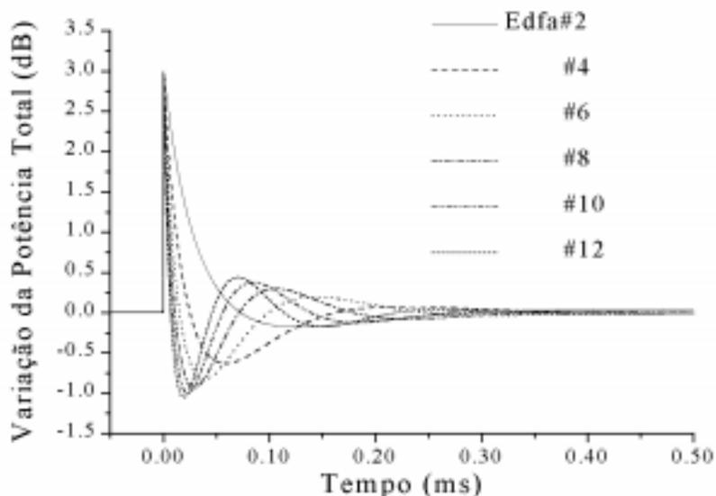
Figure 5: Variation of the total power at the output of the even-order amplifiers, when the channels no. 2, 4, 6, and 8 are added at  $t=0$  (the channels no. 1, 3, 5, and 7 were already present at  $t<0$ , and were kept in the system).
