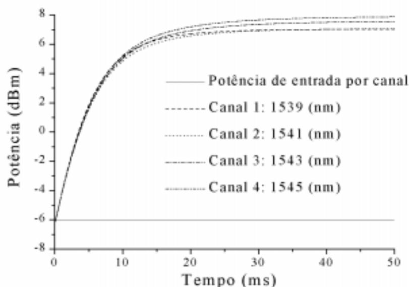
Figure 1: Temporal evolution of the output power of the channels no. 1, 2, 3, and 4, considering a single EDFA.
