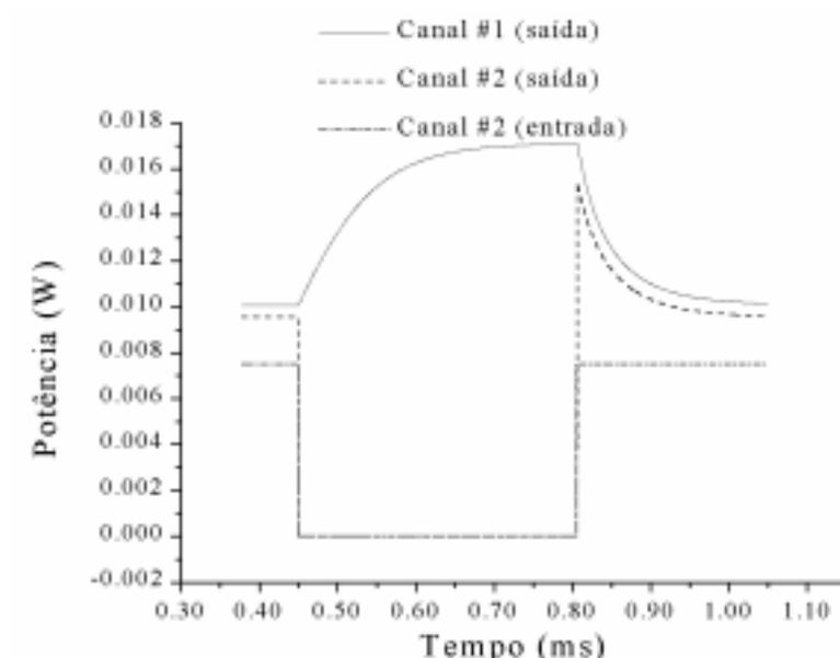
Figure 2: Output power of channels no. 1 (1539nm) and no. 2 (1541nm), when the channel no. 2 is dropped, and later added back to the system.
