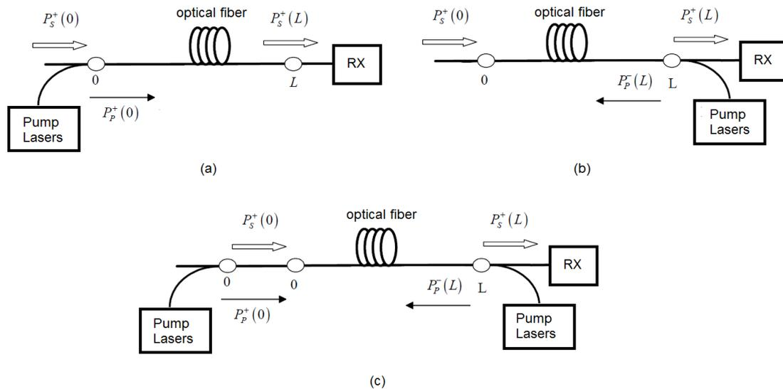
Fig. 2. Raman amplification systems with different pump configurations.
