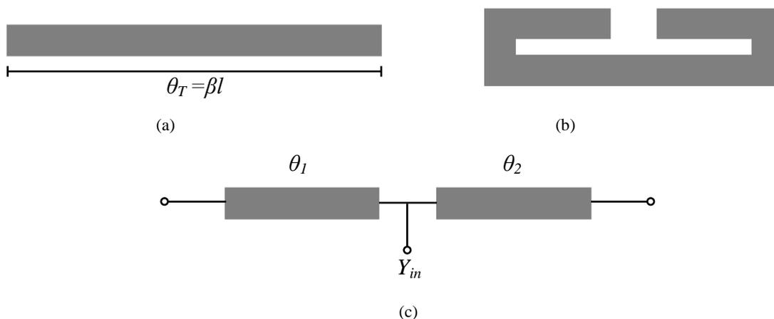
Fig. 1. (a) Straight-line resonator (b) The open loop resonator (c) Equivalent circuit of the straight-line resonator used to calculate the input admittance from any point within its length.
