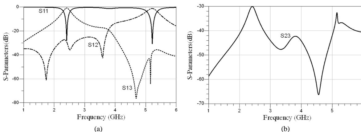
Fig. 6. S-parameters versus frequency of the proposed diplexer by using ADS (a) the return and insertion (b) the Isolation.
