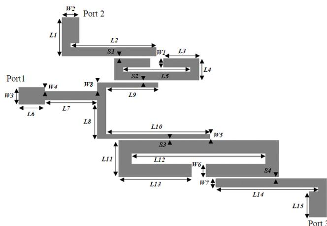
Fig.3. Physical structure and dimensions of the diplexer.
