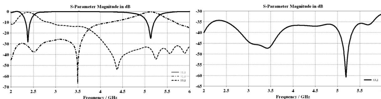
Fig. 8. The simulated results of the proposed diplexer using CST-MW.
