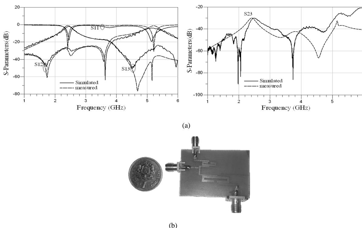
Fig. 10. (a) Simulated and measured frequency response of the fabricated filter (b) The photograph of the manufactured diplexer.
