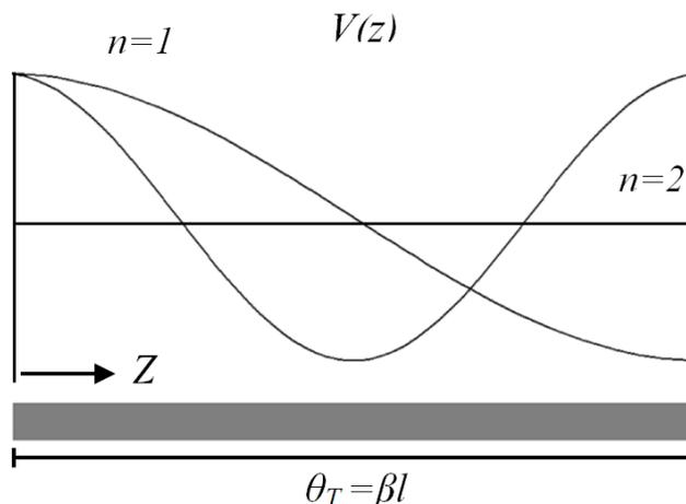
Fig. 2. Voltage distribution in a straight-line resonator.
