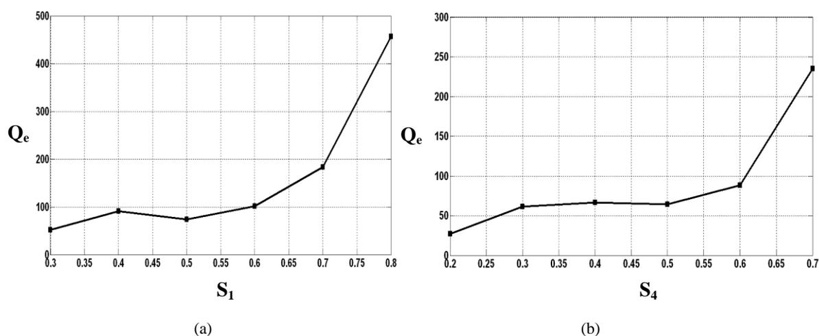
Fig. 4. Simulated external  $Q_e$  (a) by varying  $S_1$  and all the other dimensions are held constant (b) by varying  $S_4$  and all the other dimensions are held constant.
