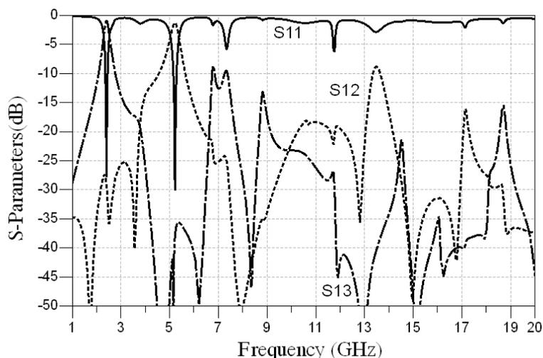
Fig. 5. Simulated frequency response of the proposed diplexer.
