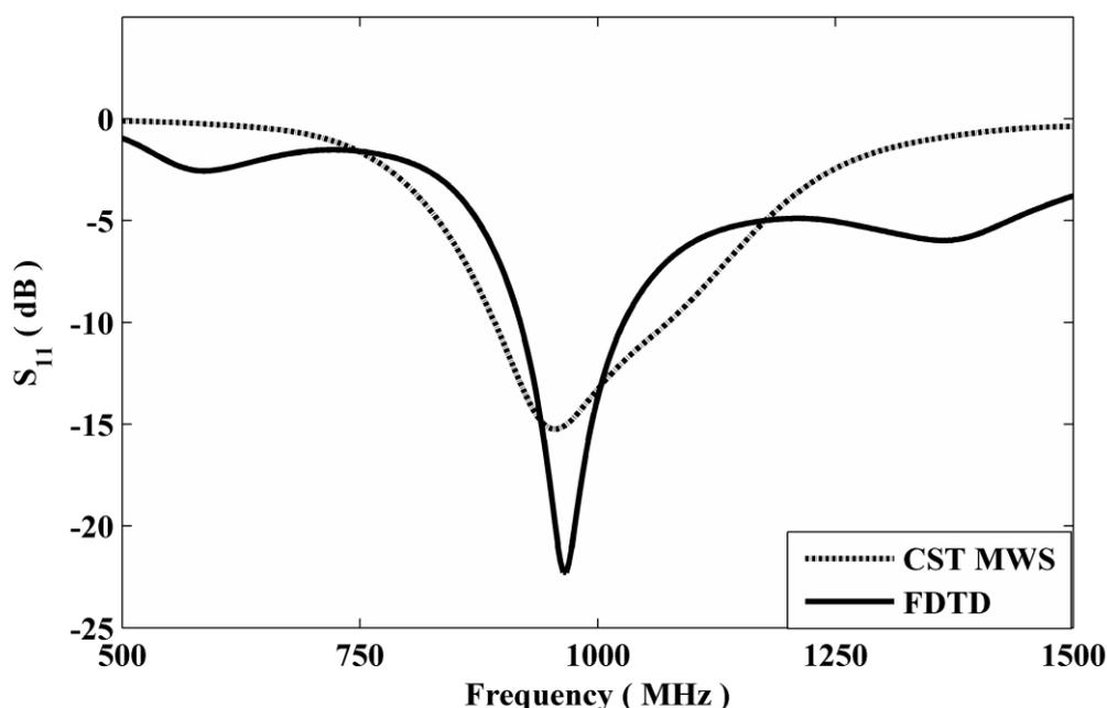
Fig. 3. Variation of  $S_{11}$  vs. Frequency of the mobile phone placed in free space.
