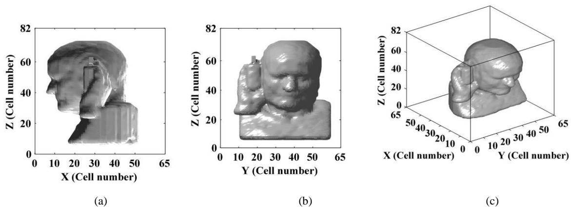
Fig. 2. (a) Sagittal plane, (b) coronal plane and (c) three-dimensional geometrical view of human head model along with hand and mobile phone.
