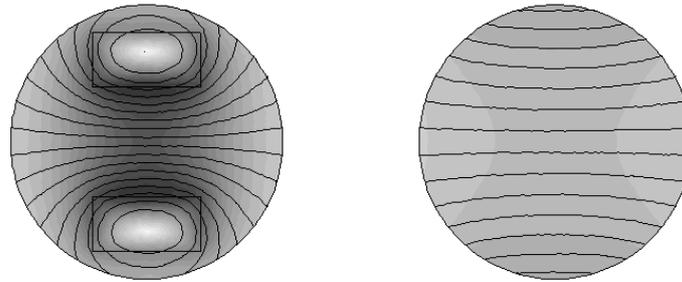
Fig. 8. Density plots of the  $B$ -field and equipotential lines for the Kelvin transformation method.
