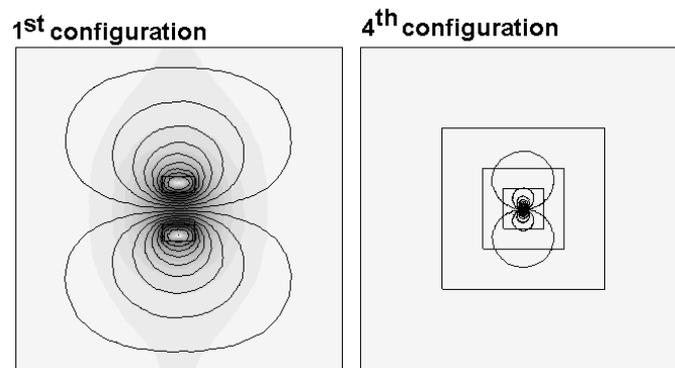
Fig. 6: Density plots of the  $\mathbf{B}$ -field and equipotential lines for simple truncation.
