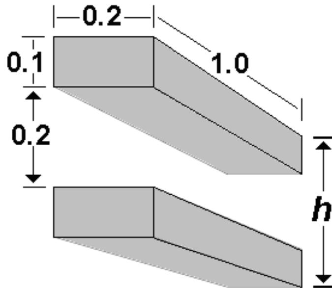
Fig. 2. Parallel rectangular busbar conductors. Dimensions in meter.
