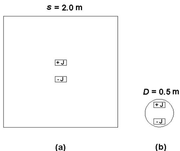
Fig. 5. Outline of the areas to be discretized. (a) Analysis by simple truncation starts with a square boundary for which the side  $s$  is 2.0 m long. (b) Analysis by the Kelvin method always uses two circles of 0.5 m diameter.
