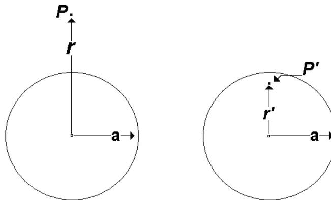
Fig. 1. Schematic representation of the Kelvin transformation.
