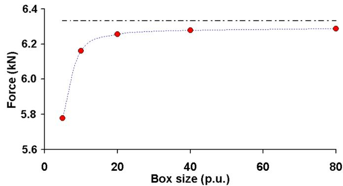
Fig. 7. The effect of increasing the boundary size on the values of computed forces.
