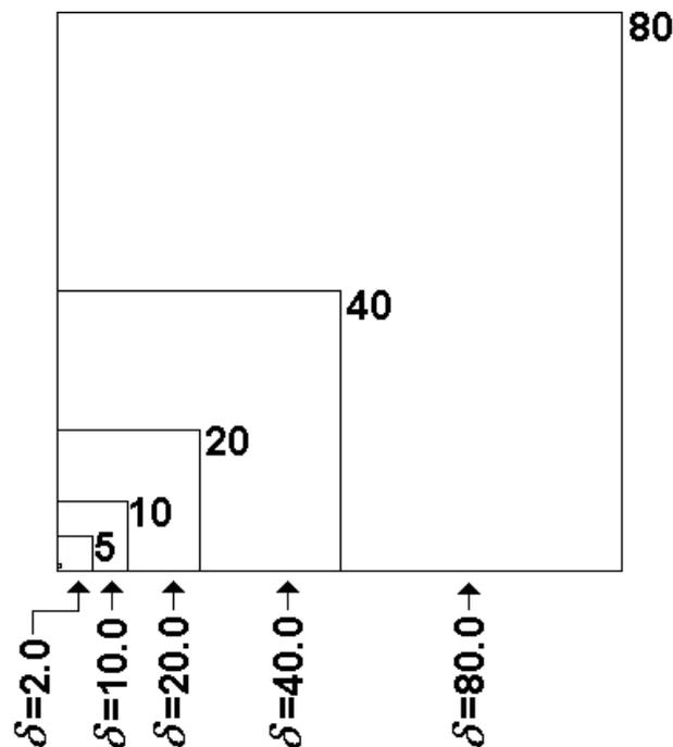
Fig. 3. Model for simple truncation; per unit values of the boundary size  $\eta$  and values in centimeter of the mesh size  $\delta$ .
