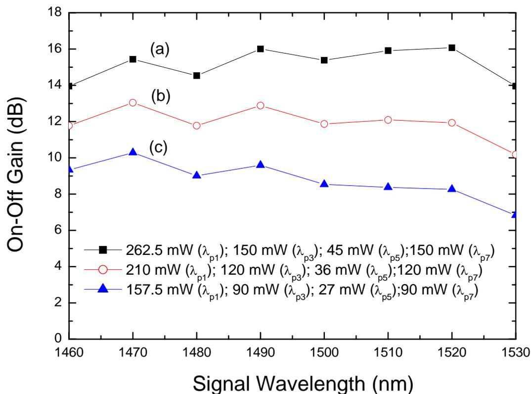
Fig. 8. On-off gain for S-band distributed Raman amplification for backward pump propagation. Four pump at wavelengths of  $\lambda_{p1}=1371.7$  nm,  $\lambda_{p3}=1389.3$  nm,  $\lambda_{p5}=1406.9$  nm and  $\lambda_{p7}=1424.5$  nm are backward propagating with respect to the signals. The power in  $\lambda_{p1}$  and  $\lambda_{p5}$  are respectively increased in 75% and reduced in 70% with respect to an equal power for all pumps of (a) 150mW; (b) 120mW; (c) 90mW.
