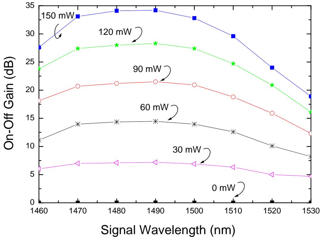
Fig.5. On-off gain for 100km distributed Raman amplification in the S-band. The pump wavelengths are centered at 1371.7nm, 1380.5nm, 1389.3nm, 1398.1nm, 1406.9nm, 1415.7nm, 1424.5nm, and 1433.3nm and are propagating backward with respect to the signals. The pumps have equal powers of 0mW, 30mW, 60mW, 90mW, 120mW and 150mW.
