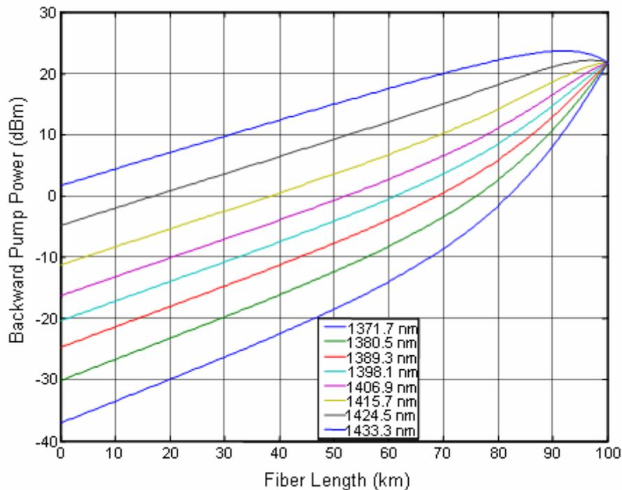
Fig.6. Backward pump power along the 100km span. All pumps are launched at span end with 150mW.
