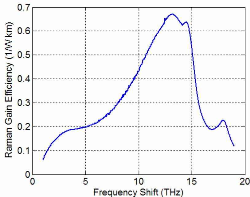
Fig. 1. Measured Raman gain efficiency curve ( $\lambda_p=1420\text{nm}$ ).
