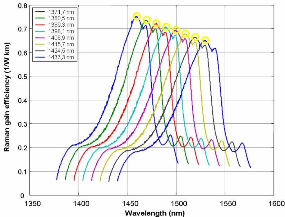
Fig.2. Raman gain curves estimated from measured data for wavelength pumps at 1371.7nm, 1380.5nm, 1389.3nm, 1398.1nm, 1406.9nm, 1415.7nm, 1424.5nm and 1433.3nm.
