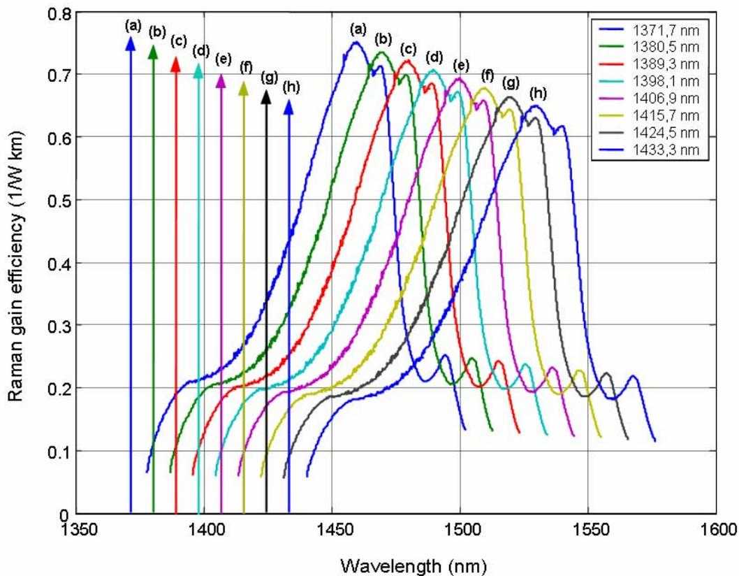
Fig. 3. Raman gain efficiency curve for eight pump wavelengths 1371.7nm, 1380.5nm, 1389.3nm, 1398.1nm, 1406.9nm, 1415.7nm, 1424.5nm and 1433.3nm. The arrows set each pump wavelength location.
