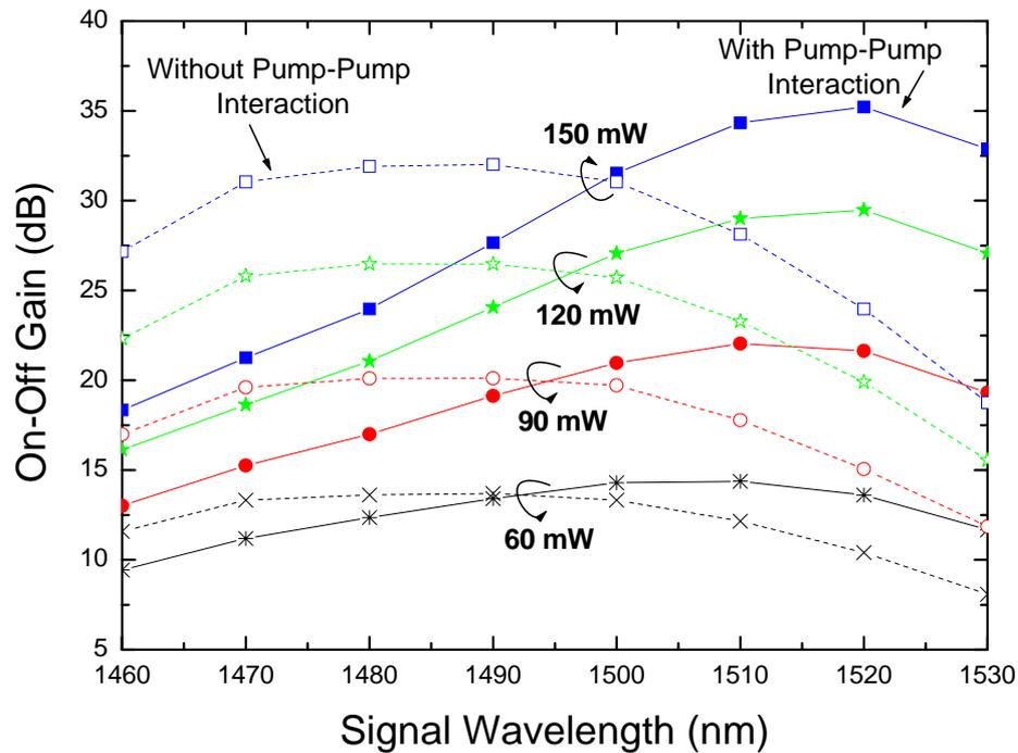
Fig. 7. On-off gain for S-band distributed Raman amplification for backward pump propagation. The pump wavelengths are centered at 1371.7nm, 1380.5nm, 1389.3nm, 1398.1nm, 1406.9nm, 1415.7nm, 1424.5nm, and 1433.3nm. The dashed lines assigns specific pump powers in the absence of pump-pump interaction and solid line assigns specific pump powers in the presence of pump-pump interaction.
