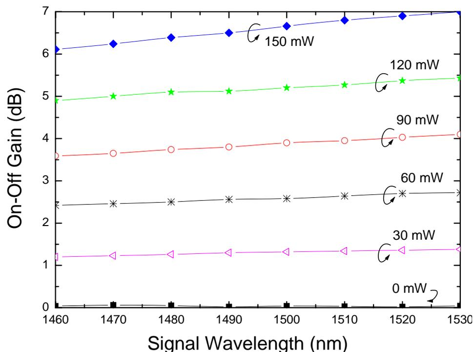
Fig. 4. On-off gain for 100km distributed Raman amplification in the S-band. The pump wavelengths are centered at 1371.7nm, 1380.5nm, 1389.3nm, 1398.1nm, 1406.9nm, 1415.7nm, 1424.5nm, and 1433.3nm and are propagating backward with respect to the signals. The pumps have equal powers of 0mW, 30mW, 60mW, 90mW, 120mW and 150mW. Only paired pump/signal contributions were accounted.
