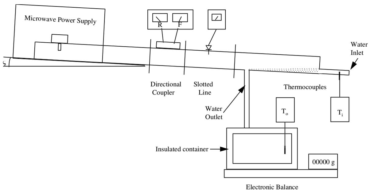
**Fig. 1.** Schematic diagram of the experimental system.
