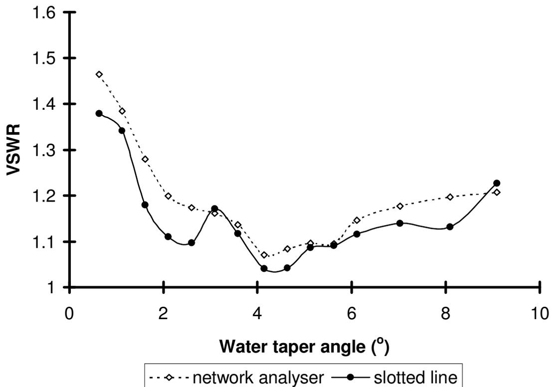
Fig. 6. VSWR measured using slotted line and network analyzer as a function of the water taper angle for water flow rate 14g/s and a power setting of 550W.
