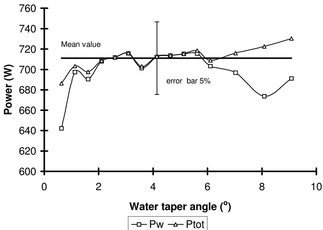
**Fig. 3.** Microwave power absorbed in the water taper and total microwave power as a function of the water taper angle for water flow rate 6 g/s and a power setting of 750 W.
