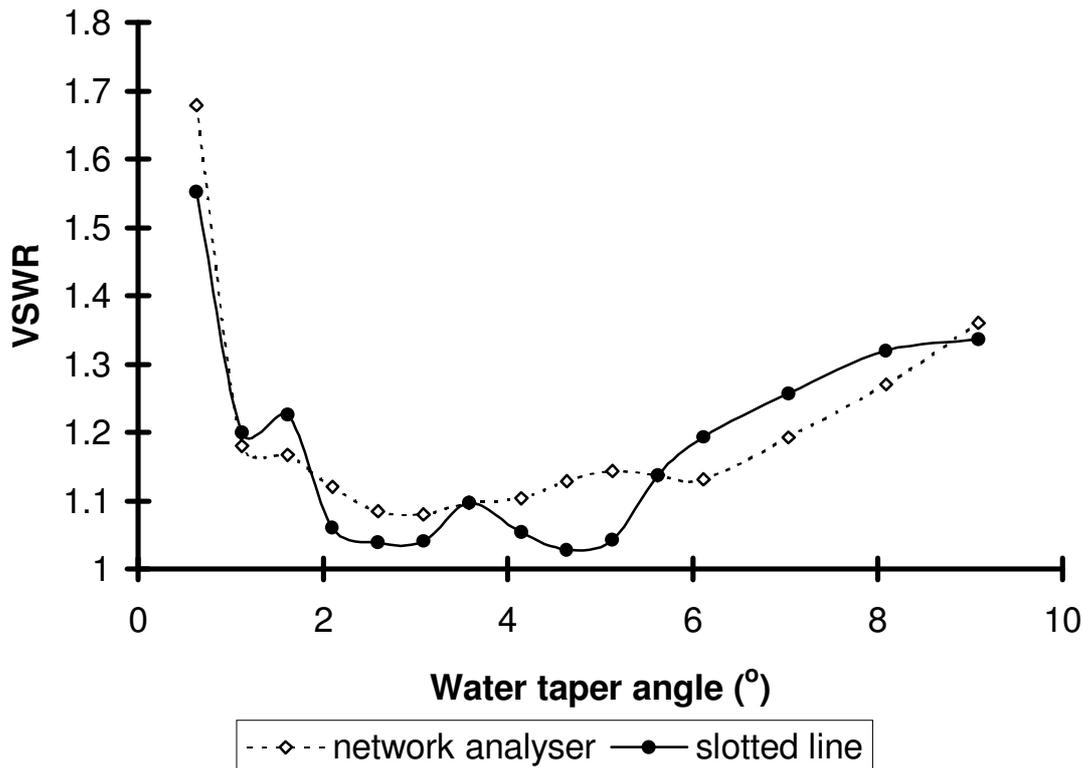
**Fig. 4.** VSWR measured using slotted line and network analyzer as a function of the water taper angle for water flow rate 6 g/s and a power setting of 750 W.
