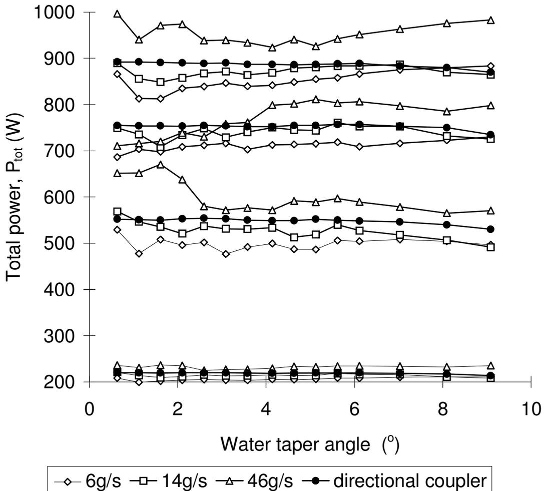
Fig. 7. Total microwave power as a function of the water taper angle for three water flow rates at various microwave power levels.
