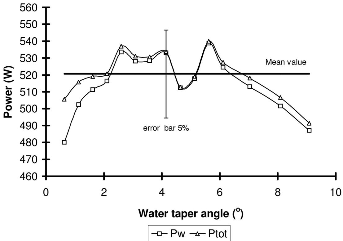
Fig. 5. Microwave power absorbed in the water taper and total microwave power as a function of the water taper angle for water flow rate 14g/s and a power setting of 550W.
