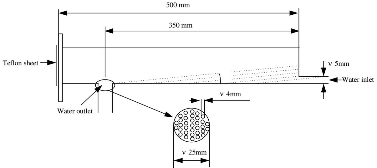
Fig. 2. Diagram of the calorimeter.
