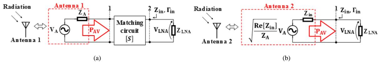
Fig. 1. Circuitual models: (a) LNA matching network - (b) directly matched LNA.
