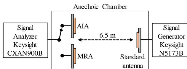
Fig. 9. Experimental setup for gain measurement.
