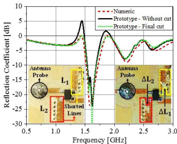
Fig. 6. Numerical vs experimental results of stabilization procedure.
