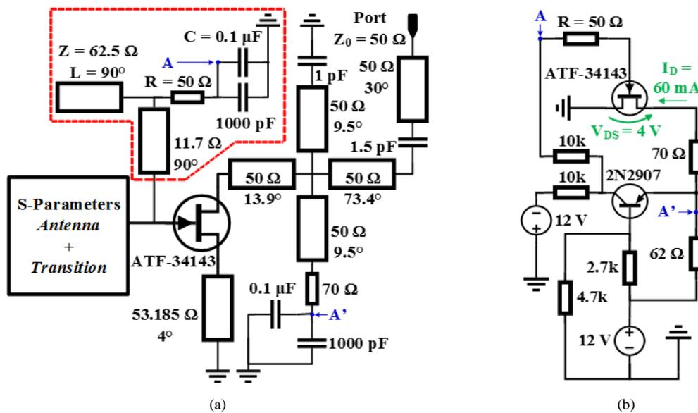
Fig. 3. Schematic: (a) RF circuit - (b) DC bias circuit.
