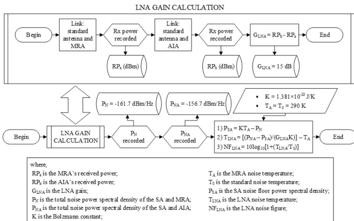
Fig 10. Flow chart describing the measures of LNA gain and NF.
