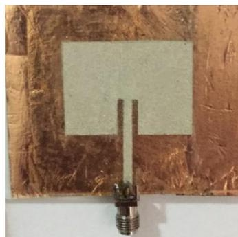
Fig. 9. Photograph of the microstrip patch antenna prototype on the glass substrate painted with the fabricated silver ink.
